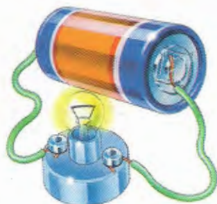
This battery (current source), wires and light bulb form a circuit.
