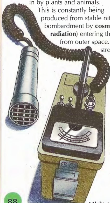
A Geiger counter , used for measuring the background count.
